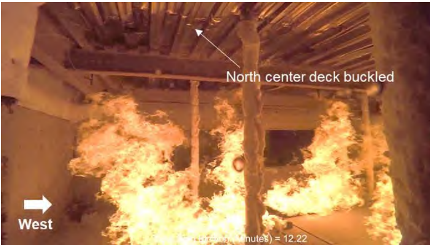
Fig. 4-25. A snapshot of the test video showing local buckling of the north steel deck at about 12 min.
