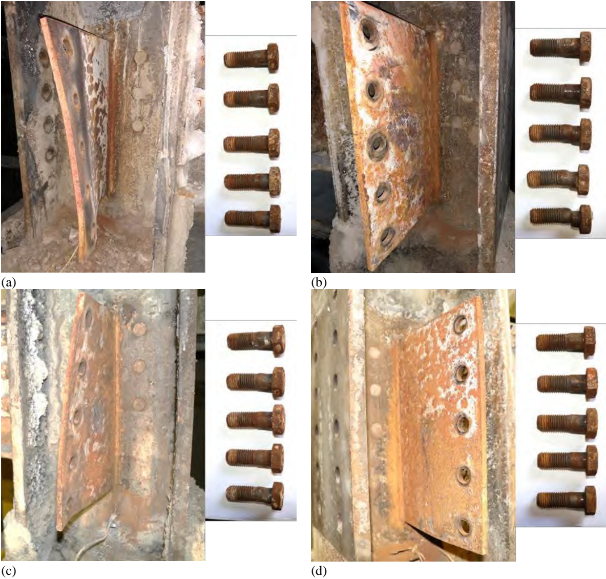
Fig. 4-48. Post-test photographs of extended shear tab (girder-to-column) connections: (a) north end of the east girder; (b) south end of the east girder; (c) north end of the west girder; (d) south end of the west girder.
