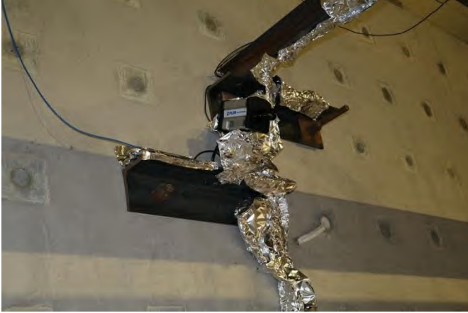
Fig. 3-8. Infrared camera mounted on the strong wall.
