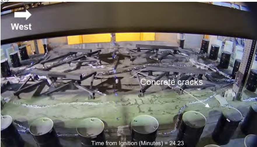
Fig. 4-26. Snapshots of the test video looking down on the top of the test floor assembly at about (a) 18 min and (b) 24 min.
