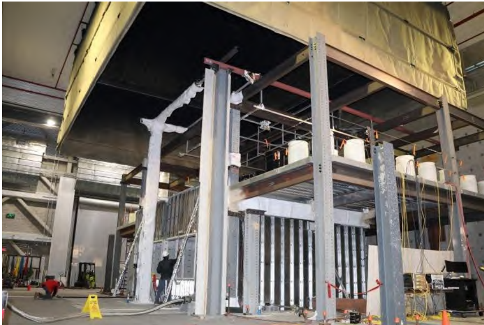
Fig. 2-2. NFRL two-story test frame prior to fire experiment.
