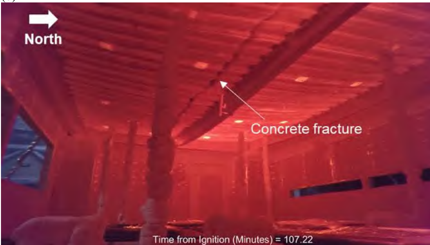
Fig. 4-24. Snapshots from the test video viewing inside the test compartment at about (a) 5 min, (b) 9 min, and (c) 107 min after the burner ignition.
